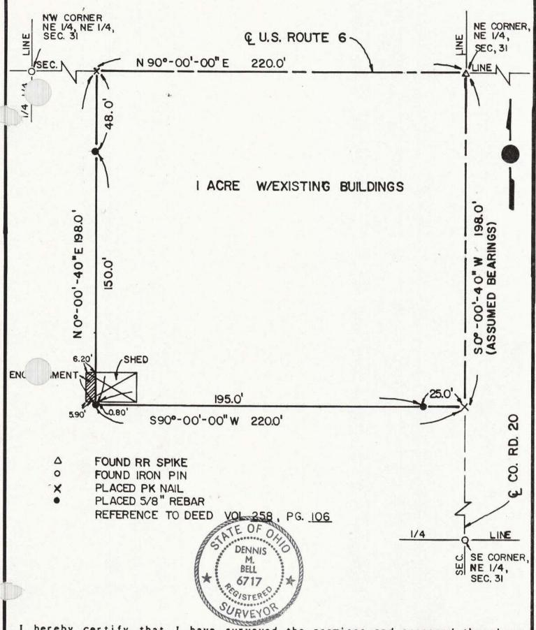
I hereby certify that I have surveyed the premises and prepared the above plat and that said plat is correct to the best of my knowledge and belief. A dimensions are shown in feet and decimal parts thereof. This survey has been recorded in Vol. Page 279 of the Williams County Record of Surveys.
